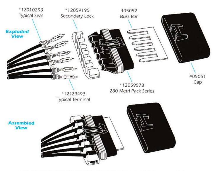
Unlimited Services Sealed Splice Pack Assembly is a connection system that allows you to eliminate multiple wire splices for a remote serviceable location on any electrical wiring harness assembly.
